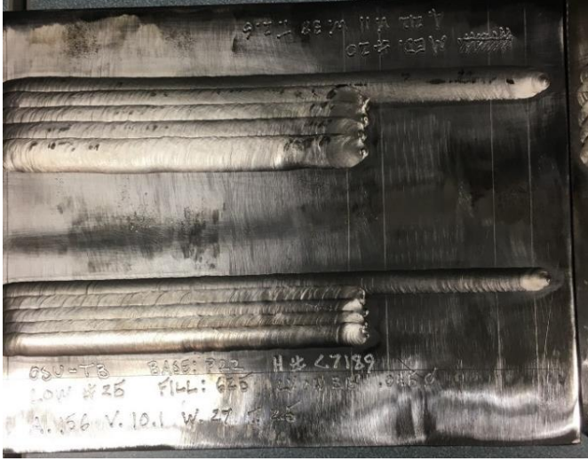
Figure 2: Test overlays used to determine TC placement.
