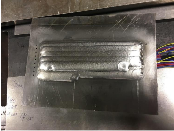
Figure 4: Completed two-layer weld overlay using the HHI welding parameters.
