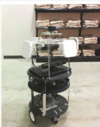
Figure 8: A Robot mounted with four RFID Antennas.
