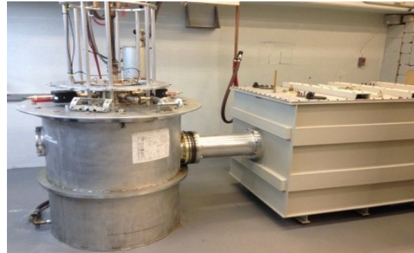
Fig. 1. 500 kV, 218 A electron gun tank (at left) connected to the 500 kV, 250 A Marx modulator (at right) in the Beam Physics Lab at Yale University.
