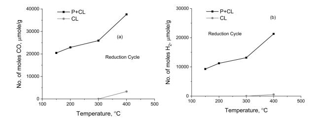
Figure 5. Number of moles of (a) CO and (b) H<sub>2</sub> formed during reduction cycle at various temperatures. P: Plasma.
