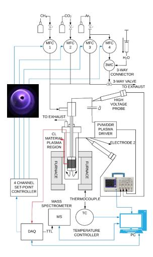
**Figure 2**. Schematic of the experimental setup (Color lines are seen in the online version only). A bottom view picture of the plasma is shown on the left.
