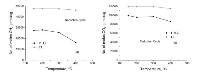
Figure 5. Number of moles of (a) CH<sub>4</sub> and (b) CO<sub>2</sub> consumed during reduction cycle.The H<sub>2</sub> generated by water splitting during oxidation cycle at different temperatures is plotted inError! Reference source not found.. The experiments without plasma showed hydrogen
