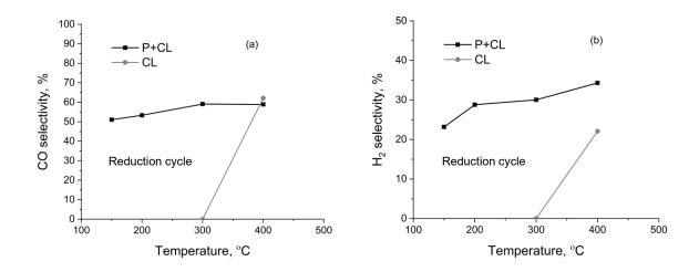
Figure 8. Selectivity (a) CO and (b) H<sub>2</sub> vs. temperature.
