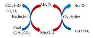
Figure 1. Chemical looping reforming process. (Color lines are seen in online version only).
