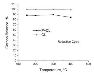
Figure 6. Estimated carbon balance for the experiments at different temperatures.
