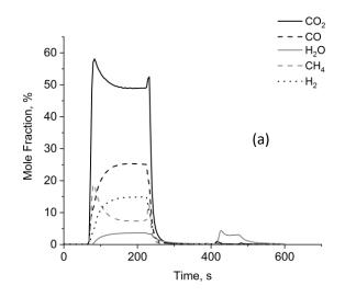
**Figure 4**. Measured time resolved species mole fraction after flow over the nanomaterial during a reduction/oxidation (redox) cycle, at 1000 °C, 1 atm pressure.
