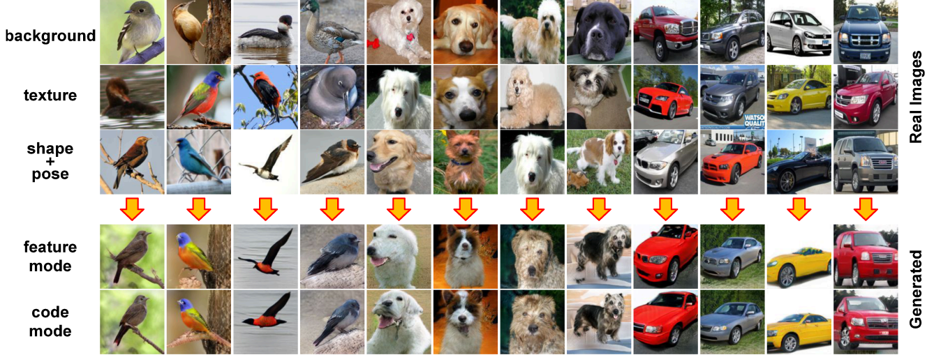
Figure 3: Comparison between code mode & feature mode. Rows 1-3 are real reference images, in which we extract background b , texture c , and shape+pose p & z , respectively. Rows 4-5 are MixNMatch’s feature mode (which accurately preserves original shape information) and code mode (which preserves shape information at a semantic level) generations.
