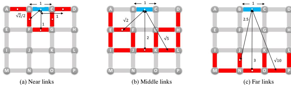
Fig. 2. Examples of link-center distance categorization in  $4 \times 4$  mesh network model with a uniform distance between adjacent nodes.
