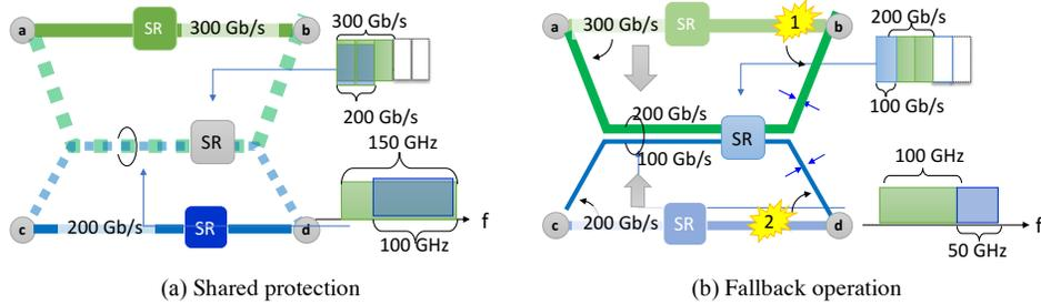
Fig. 1. Shared protection with fallback in a translucent EON.
