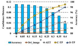
Fig. 8: The relationship between confidence distance and model accuracy with weight error  $\boldsymbol{\sigma}$
