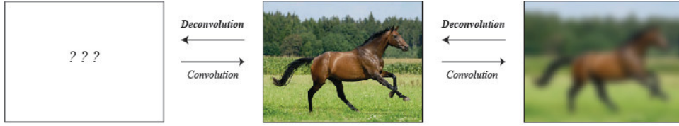
Figure 1: Performing convolution on this real world image using a correlative filter, such as a Gaussian kernel, adds correlations to the resulting image, which makes object recognition more difficult. The process of removing this blur is called deconvolution . What if, however, what we saw as the real world image was itself the result of some unknown correlative filter, which has made recognition more difficult? Our proposed network deconvolution operation can decorrelate underlying image features which allows neural networks to perform better.
