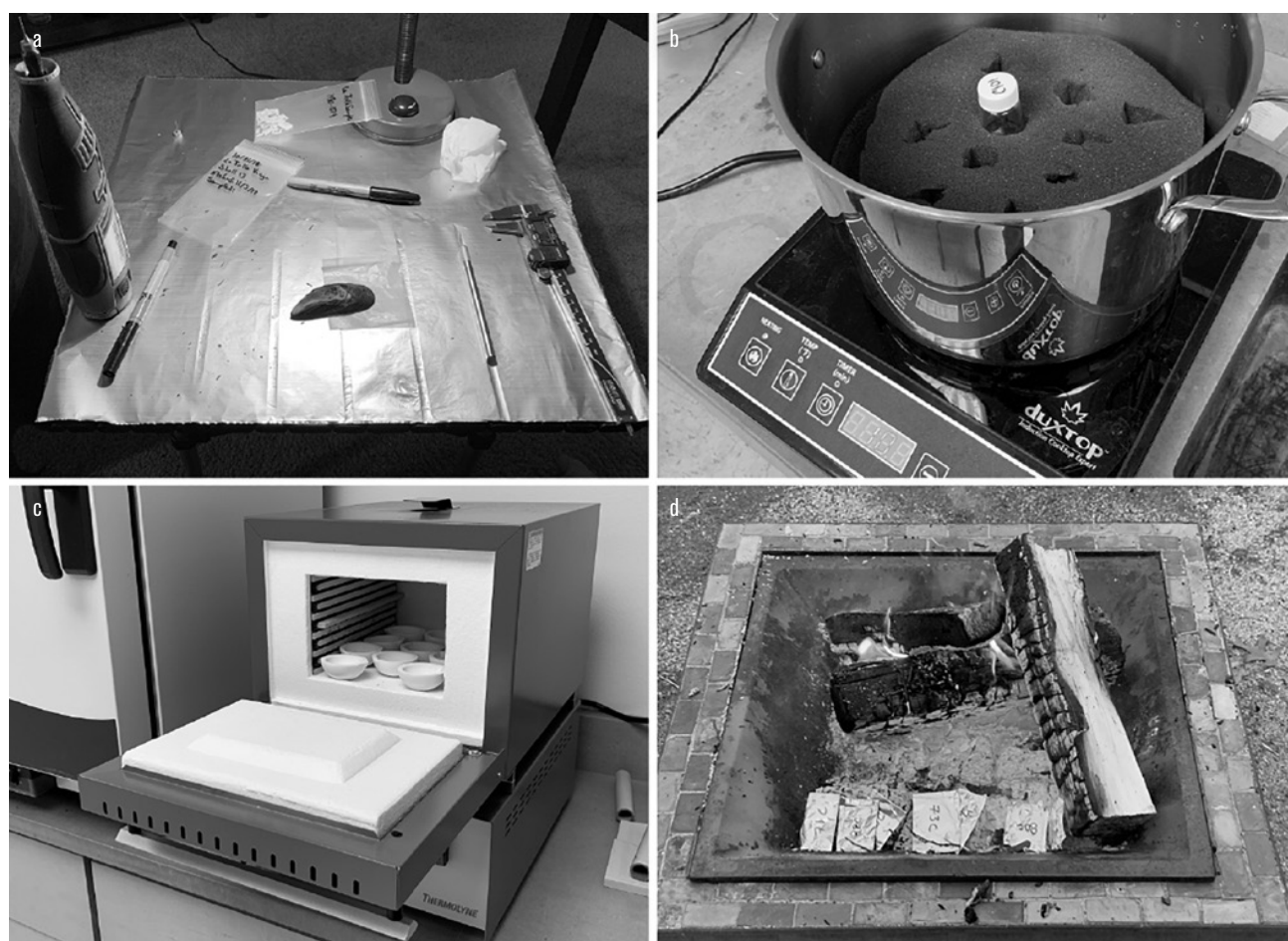
Figure 3. Images representing the primary experimental steps: (a) a characteristic sample drilling kit, including calipers and a Dremel tool; (b) an induction cooktop used for boiling shell powder in scintillation vials; (c) a muffle furnace with samples in ceramic crucibles; and (d) a campfire with samples in foil envelopes being heated by coals.
