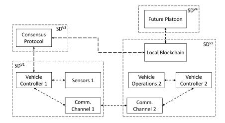
Figure 6. Cyber Only Blockchain Information Flow Diagram
