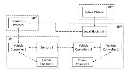
Figure 7. Physical Only Blockchain Information Flow Diagram
