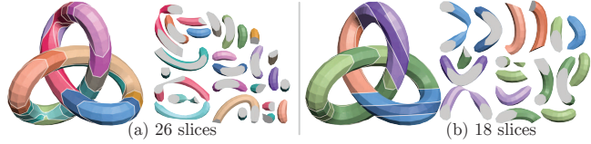
Fig. 8. Using LDHF blocks (b) instead of DHF ones (a) keeping the rest of the process the same introduces significantly fewer slices (18 vs 26 in this example), and reduces the prevalence of thin slices.
