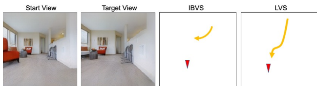
Fig. 6. Visualization of a test case where correspondence is missing during navigation. Given the start view and goal view, the robot should move right then turn left. Using IBVS, robot stops due to loss of FOV overlap. Using LVS, robot is able to reach the goal.
