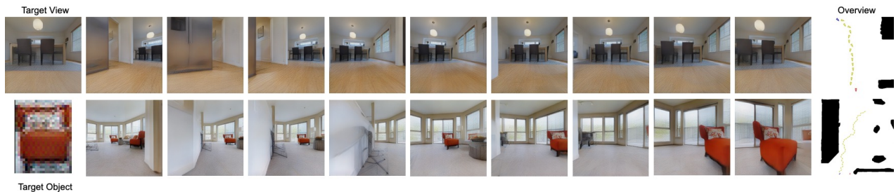
Fig. 5. Examples of a robot driving to a view (first row) and driving to an object (second row). The first column shows the target view and the target object. The last column is the overview of the two trials. Between them are the observations along the driving.
