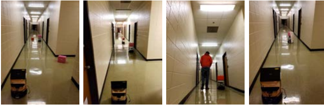
Fig. 6: Robustness tests involving background noise via similarly colored boxes on the floor, low ambient light, human sharing the space, and observed robot is partially occluded.
