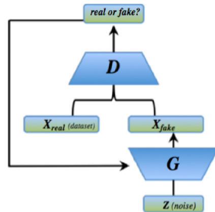
Fig. 1. Illustration of competing neural networks, discriminator D and generator G, in Generative Adversarial Networks (GAN) technique.
