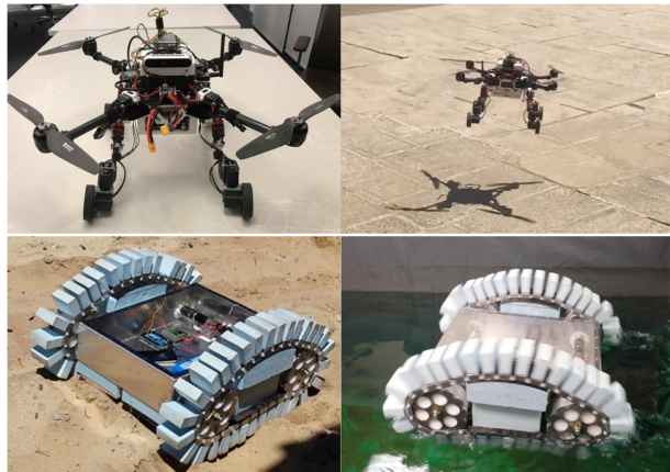
Fig. 1. Top Row: A "Drivocopter" Drone (developed by the authors) which can fly and drive. Video of operation can be accessed at https://www.youtube.com/watch?v=QZyuvXfifvQ . Bottom Row: "Ambot" Amphibious Robot [1] capable of ground and marine locomotion.
