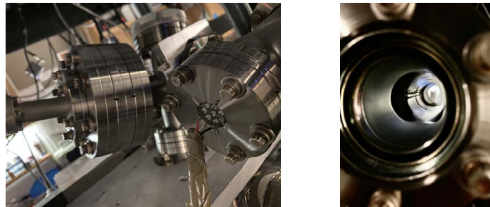
Figure A.6: The side feedthrough (left) and shutter cables (right) viewed from the transverse viewport.
