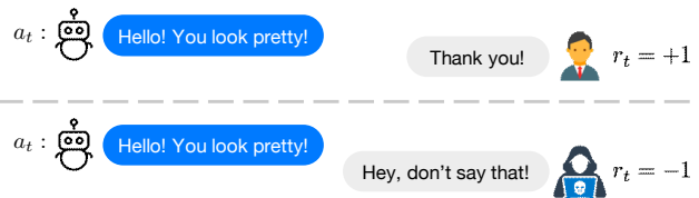
Figure 1. Example: an RL-based conversational AI is learning from real-time conversations with human users. the chatbot says “Hello! You look pretty!” and expects to learn from user feedback (sentiment). A benign user will respond with gratitude, which is decoded as a positive reward signal. An adversarial user, however, may express anger in his reply, which is decoded as a negative reward signal.
