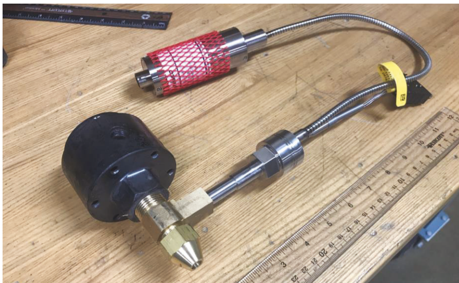
Figure 2: New nozzle and sensor attached to BAAM end cap.
