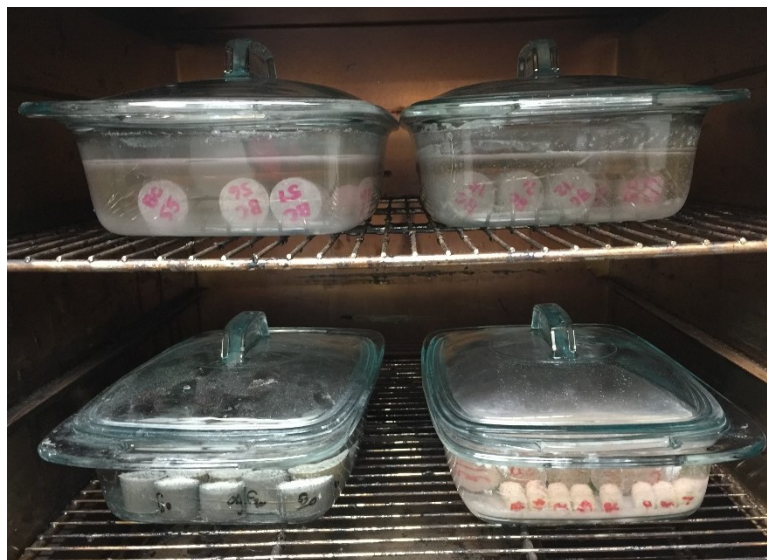
Figure 2: Conditioning of GFRP bars
