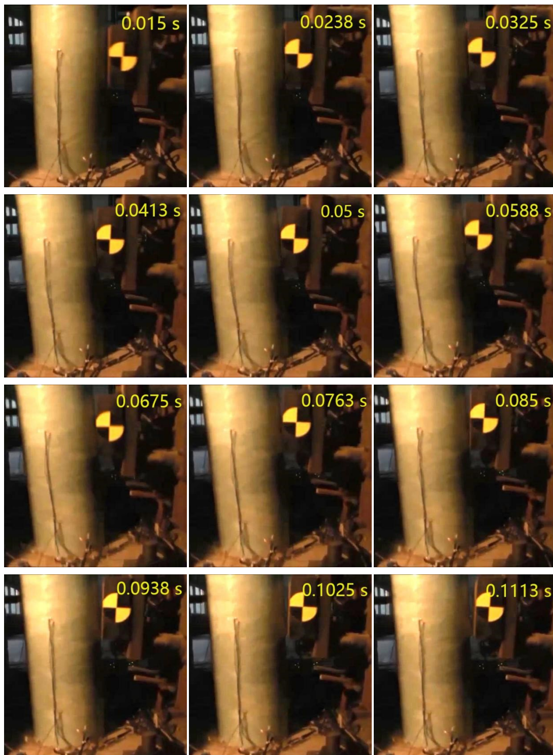
Fig.6 Typical impact failure process (i.e. D7- II)
