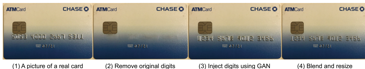
Figure 3: Fugazi’s basic process for creating fake card images. The process uses four steps and combines traditional image manipulation techniques with deep learning.
