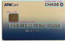
Figure 14: A BIN inconsistent fake card image caught by our BIN consistency and expectation check. The card shown in the image starts with a 4 and should thus have the Visa logo. The BIN (first 6 digits) of the card is also not from Chase, and thus, a Chase logo should not be present. Our check detects both inconsistencies, showing that it would flag such a card as fake.
