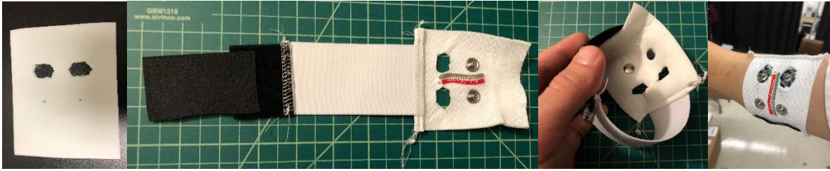
Figure 5. Construction of armband for dual-channel sEMG signal collection of the same arm muscle.
