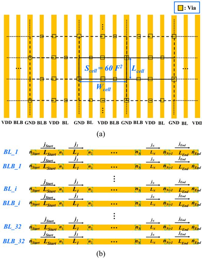
Fig. 4. (a) Interconnect segment array of an FinFET SRAM, with periodic cells shown, and (b) 32 pairs of interconnect segment arrays used for the calculation (32 columns of BL/BLB), where  $L_{Start}$  and  $L_{End}$  represent the interconnect lengths from the array to the precharge and write drivers, respectively.
