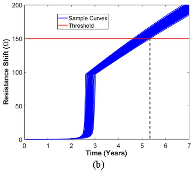
Fig. 13. (a) Variation of the hydrostatic stress distribution on a sample BL at 3.5 years (Left: Precharge side, Right: write drive side), and (b) variation of the overall resistance shift of a sample BL. The input data distribution has a mean duty cycle of 10%.
