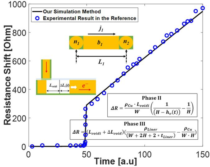
Fig. 2. Resistance trace of interconnect with  $L_1 = 250\mu\text{m}$ ,  $j_1 = 2.0 \times 10^7 \text{ A/m}^2$  [23].
