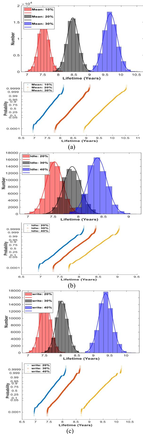
Fig. 14. Histogram and cumulative distribution plots of (a) effect of input data distribution's mean probability on the lifetime distribution, with read (60%), write (20%), and idle (20%) percentages unchanged, (b) effect of the idle percentage on the lifetime distribution, with the relative percentage ratio between read and write unchanged, and (c) effect of the write percentage on the lifetime distribution, with the idle (20%) percentage unchanged.
