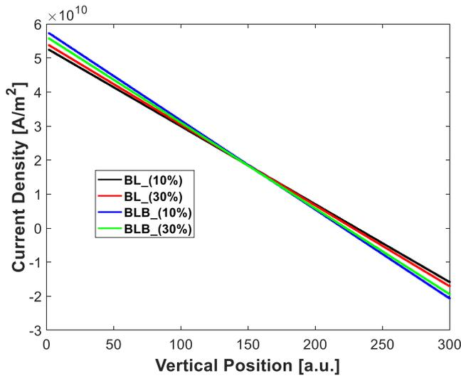
Fig. 12. An example of current density over BL/BLB in the first column, with different input data (mean signal probabilities of 10%, and 30%).
