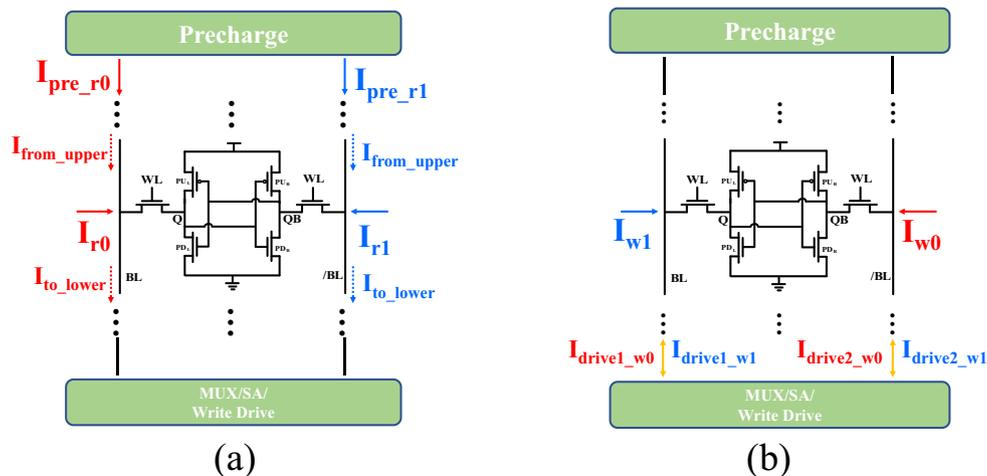
Fig. 5. Currents related to the EM calculation during (a) r0 and r1, and during (b) w0 and w1.
