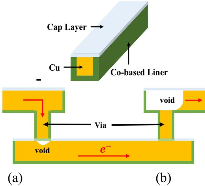
Fig. 1. (a) Cu dual damascene conductor structure, where the trench is lined with a Cobalt-based liner and the Cu is capped with either a dielectric or metallic layer. (b) A Cu wire connected with a via-below (left) and a via-above (right) [11].
