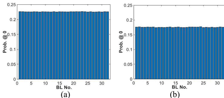
Fig. 10. Extracted probability that BLs are 0, with different input data (mean of distributions at (a) 10% and (b) 30%).
