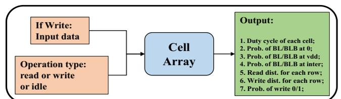
Fig. 8. Simulation flow for activity extraction.
