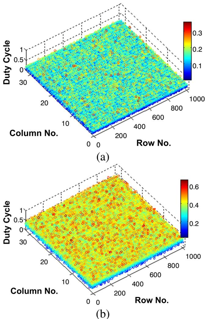
Fig. 9. Extracted duty cycle distribution with different input data (mean of distributions at (a) 10% and (b) 30%).
