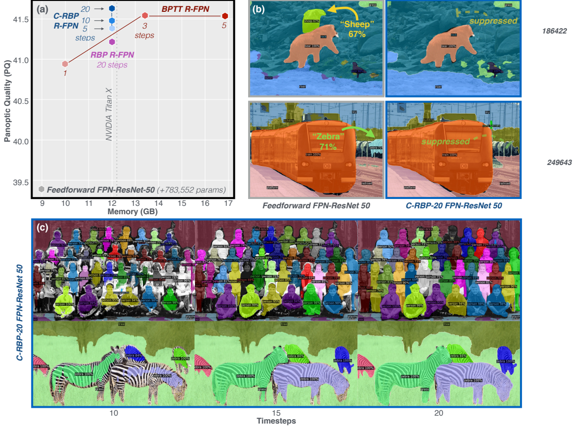
Figure 3: C-RBP trained recurrent vision models outperform the feedforward standard on MS-COCO Panoptic Segmentation despite using nearly 800K fewer parameters. (a) Performance of our recurrent FPN-ResNet 50 trained with C-RBP improves when trained with more steps of processing, despite remaining constant in its memory footprint. (b) Recurrent processing refines instance segmentations and controls false detections exhibited by the FPN-ResNet 50 (additional examples in SI). (c) Panoptic segmentation timecourses for an FPN-ResNet 50 trained with C-RBP for 20 steps.
