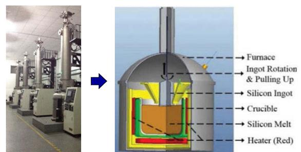
Fig. 1. A schematic of a crystal growth furnace network: the furnaces (left) and its internal structure (redrawn with authors' permission) [1]
