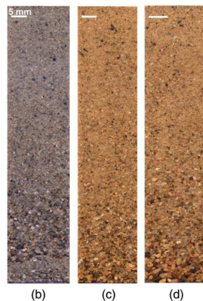
Fig. 13. Specimen C: (a) verification PSDs; (b) field; (c) field-repeat; and (d) lab photographed FieldSed sides.
