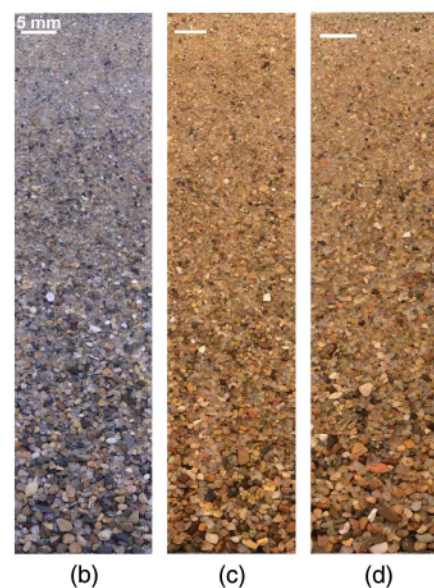
Fig. 11. Specimen A: (a) verification PSDs; (b) field; (c) field-repeat; and (d) lab photographed FieldSed sides.
