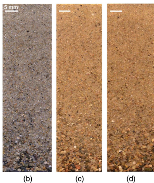
Fig. 14. Specimen D: (a) verification PSDs; (b) field; (c) field-repeat; and (d) lab photographed FieldSed sides.
