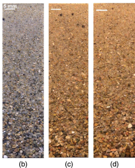
Fig. 12. Specimen B: (a) verification PSDs; (b) field; (c) field-repeat; and (d) lab photographed FieldSed sides.
