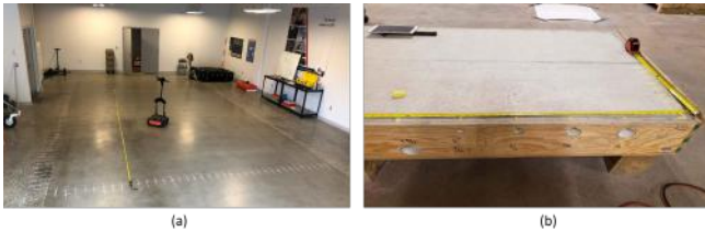
Fig. 3. (a) Test pit in GSSI's garage, multiple targets buried underneath the surface. (b) Test slab in GSSI's slab room, multiple utility pipes inserted in the slab.
