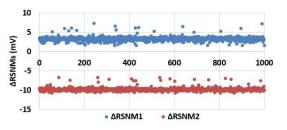
Figure 7: The read noise margin changes after 60 months usage for 1000 monte carlo SRAM cell instances with process variations.
