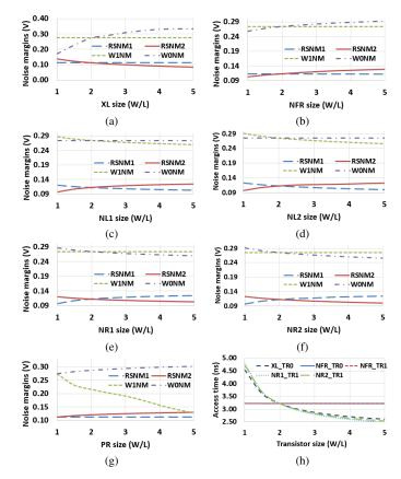
Figure 5: Noise margins of the SRAM cell versus the sizes of (a) XL (b) NFR (c) NL1 (d) NL2 (e) NR1 (f) NR2 (g) PR. (h) Access time of the SRAM cell versus the transistor sizes.
