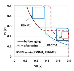
Figure 3: The butterfly curve of a 10T ST SRAM cell indicating RSNM before and after aging.
