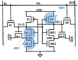
Figure 2: 10T ST SRAM cell.
