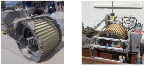
Figure 1: Tactile wheel mounted on a rover (left) and with a data-taking test cart (right). The pressure sensor array wraps around the wheel and is covered with a yellow protective layer of Kevlar.
