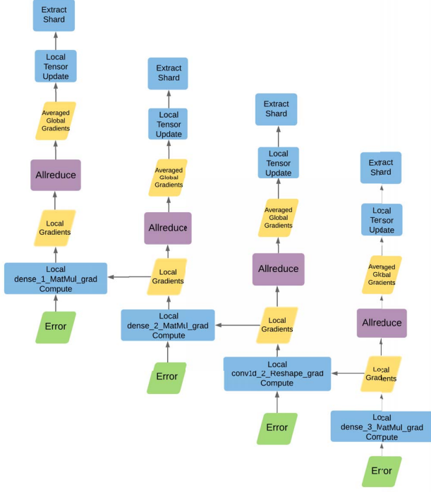
Fig. 3: Example of fine-grain sharding during back-propagation, including the pipeline between the shards.
