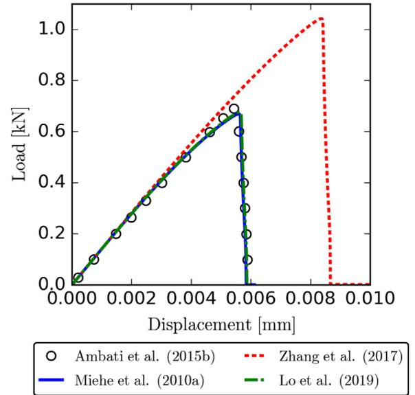
**Fig. B.2.** Load–displacement curves for single edge notched tension test. The solid and dashed lines depict the numerical results obtained from phase field model based on the corresponding strain energy decomposition schemes. The black circular maker represents the benchmark solution digitized from Figure 9 of [34].
