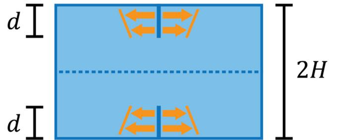
**Fig. C.1.** Double edge cracks through finite slabs with  $H$  in width and  $d$  in crack length. The yellow arrows indicate applied loading on the crack surface that leads to crack opening. The dashed line of symmetry represents the free slip surface at the base of the glacier.
