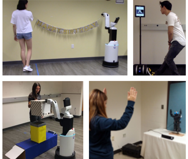
Fig. 1. Examples of robots engaging in proximate HRT from our prior work (clockwise from top left): collaboratively hanging a banner [51], engaging in rehabilitation exercises [52], implicitly learning from a human [18], and stacking boxes [32]. These platforms act in shared spaces with people, and need to be able to team fluently with their human partners for successful interactions.
