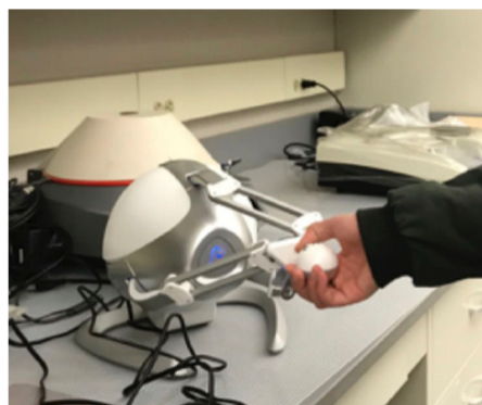
Figure 1. Operation of the Novint Falcon® based Rubber Emulator.
