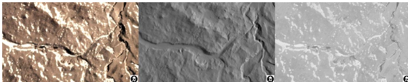
Figure 2: Image processing example. A. shows the original 3-band raster from Planet Labs. B. shows the LIDAR 3 meter DEM. C. shows the final terrain-corrected image with topographical shading removed from a summed reflectance raster calculated from A.
