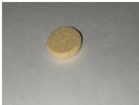
FIGURE 12: COMPLETED PRINTLET OD 10 MM DIAMETER, 3 MM HEIGHT
