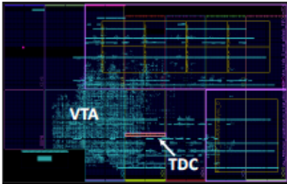
Fig. 2: Floorplan (horizontal view) for the ZC706 board showing the location of the victim VTA and attacker TDC modules.
