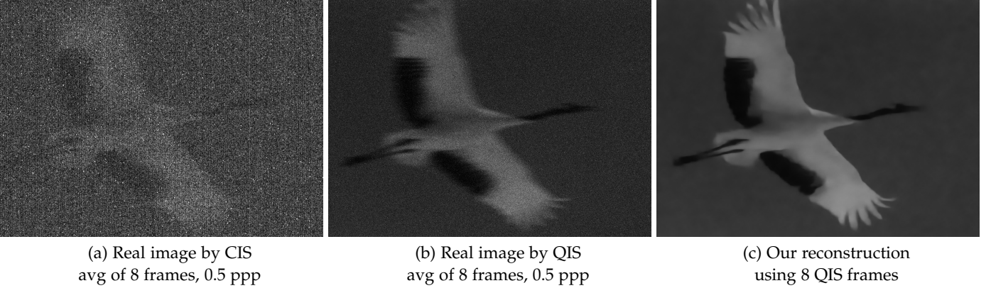
Fig. 1. Goal of this paper. The images above are the real captures by a CMOS Image Sensor (CIS) and a QIS prototype [6] at the same photon level of 0.5 photons per pixel (ppp) per frame. The strong shot noise and read noise of CIS makes signal acquisition difficult, whereas the QIS can obtain a better image. Using the proposed method, we are able to reconstruct images with dynamic content.
