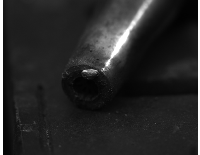
FIGURE 12. Photograph of the tip after test 2603. Dross adhered to the torch tip.
