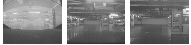
Figure 15: Three kinds of camera images dumped from GPU memory. Left one is the fisheye image; middle one is the main image and right one is the narrow image. We found that the lane detection is based on the main image.
