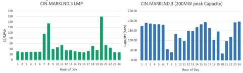
**Fig.4.** Power price (\$/MWh) (left) and resulting resource capacity for a 200 megawatt datacenter (right), using constant cost purchase approach. Exemplar 24-hour day from MISO January 9, 2018, CIN.MarkInd grid node.
