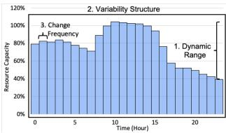
**Fig.3.** Modeled dimensions of capacity variation include (1) dynamic range, (2) variability structure and (3) change frequency (temporal granularity) on a time-sequence of datacenter capacity from Figure 2(b).
