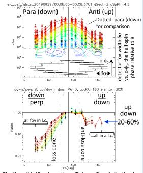
Finding #1 (Backscatter @ Low Precipitation) The up and down fluxes tend to become comparable. Their ratio typically becomes >20% and often >60%. Ratios of r~1 are also an attribute of noise  $(\delta r/r^2)/\sqrt{N}$ , where N= # of counts). Large ratios (near 1) are often seen as energy increases and counts become low, but this is not always physical. Proper statistics must be applied, as done here.
