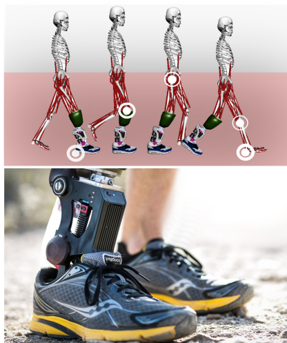
Figure 1: Top: Probabilistic modeling predicts upcoming motion and joint stresses. Circles indicate high-impact joints. Bottom: Control signals for our robotic ankle prosthesis are generated in order to minimize joint stress.
