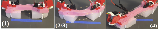
Fig. 5: The steps for the left turning motion of the soft robot (right side is the front part of the robot).
