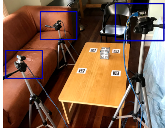
Figure 3: The experiment was designed to evaluate complex, three dimensional contact. A cube was tossed against the planar ground, producing impacts and both sticking and sliding frictional contact. Cube position and orientation are tracked by three cameras, outlined in blue.
