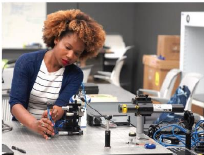
LaserTech student Genell Hoechstetter mounts a photodiode to an optical breadboard as part of her studies on how to align a pinhole spatial filter to a focused beam of light.
