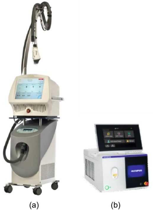
Figure 22. (a) Dual 1550/1927 nm, erbium/thulium fiber laser used in dermatology for fractional skin resurfacing (wrinkle removal). (b) Thulium fiber laser at 1940 nm used in urology for treatment of kidney stones.
