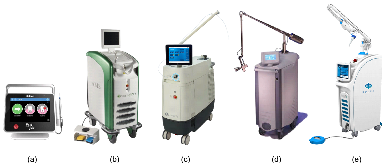
Figure 21. (a) Small, tablet-size 980 nm diode laser used in soft tissue dental procedures. (b) High-power “Greenlight” KTP visible laser at 532 nm used in urology for vaporization of the prostate gland. (c) High-power Ho:YAG infrared laser at 2120 nm with flexible fiber-optic delivery system for endoscopic procedures in gastroenterology and urology. (d) High-power Er:YAG mid-IR laser at 2940 nm with an articulated arm and scanning system, used in dermatology for cosmetic skin resurfacing. (e) High-power CO 2 mid-IR laser at 9,600 nm with an articulated arm, used in dentistry for removal of dental decay.
