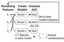
Fig. 3: Backwards elimination with n feature groups remaining. First, n models are created with 1 of the feature groups omitted, then the models are evaluated based on their AUC. The feature groups contained within the best performing model are used for the next iteration.
