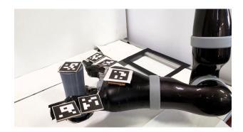
Fig. 4: Real world test setup. The ArUco markers were used to measure the finger, object and palm location and the box was used to tell if grasps were successful or not.
