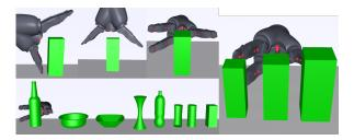
Fig. 1: Top left: Hand orientations: rotated, top down and normal. Bottom left: Shapes: tall bottle, rounded bowl, rectangular bowl, hourglass, short bottle, vase, cylinder and box. All shapes shown are medium sized. Right: The three sizes; all shapes have three sizes with these relative proportions.
