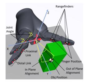
Fig. 2: All locations are relative to a coordinate system centered on the palm. The object position is the center of the object. We place two range finders on each link and five on the palm, shown as red dots in this image.
