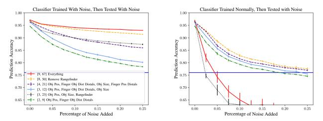
Fig. 6: Left: Testing and training with noise. Right: Just testing with noise. Legend policies ordered by feature groups and length of grasp metrics. The blue horizontal line in each plot indicates the accuracy of an "assumed bad grasp" policy.
