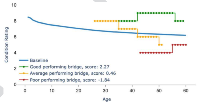
Fig. 3. Comparison of good, average, and poor performing bridges against blue national baseline. x -axis is bridge age and y -axis is bridge condition.
