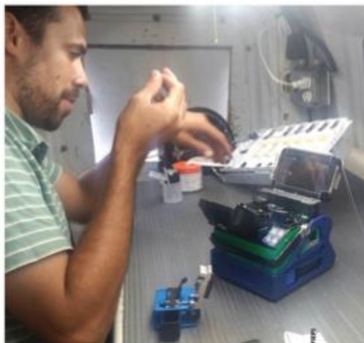
PRPI student Marcos Santini splices an optical fiber damaged during Hurricane Maria.
