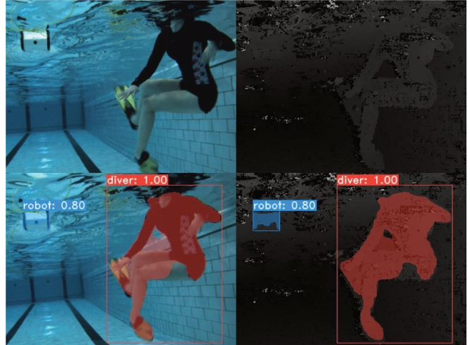
Fig. 1: Four levels of scene understanding in underwater human-robot collaborative missions, shown top-to-bottom, left-to-right: observation with no understanding (RGB image), distance-aware observation without scene understanding (depth estimation), instance-aware scene understanding (instance segmentation), and depth-instance-aware scene understanding (depth-instance segmentation). We propose a depth-instance-aware approach for obstacle avoidance.
